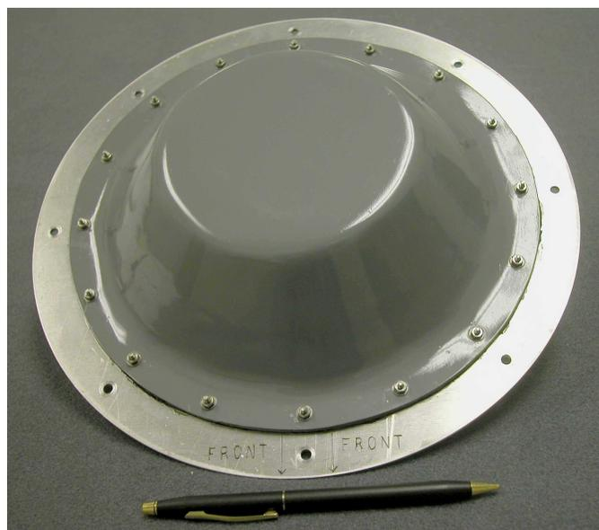
Fig. 12. A brassboard model of the circular beam-steering array.
